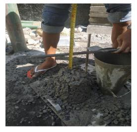
Source : Lab Research Results, 2020 Figure 5. Slump Test
