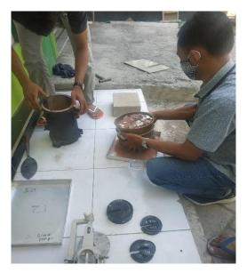
*Source : Lab Research Results, 2020* Figure 3. Ceramic waste powder sieve process
