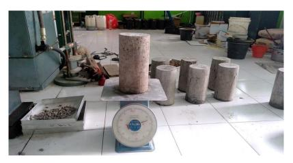
Source : Lab Research Results, 2020 Figure 6. Weighing the test object
