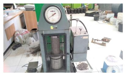
Source : Lab Research Results, 2020 Figure 7. Concrete compressive strength test
