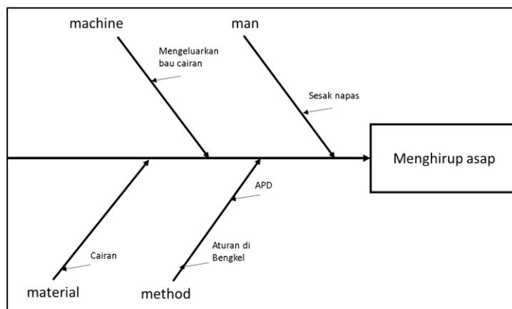
Gambar 4 Diagram Fishbone Menghirup Asap
