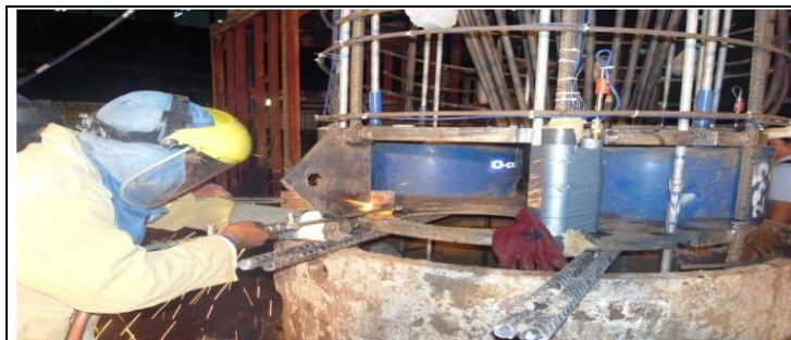
Figure 2. Hydraulic Jack Osterberg Cell.
