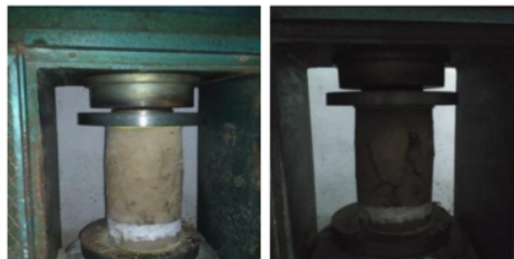
Figure 4. Compressive Strength Test of Concrete
