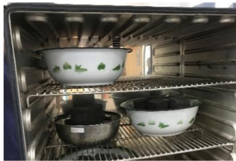
Figure 3. Mortar Cubes in the Drying Oven
