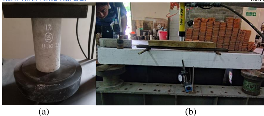
Figure 3. (a) Compression Strength Testing (b) Beam Test Setting
